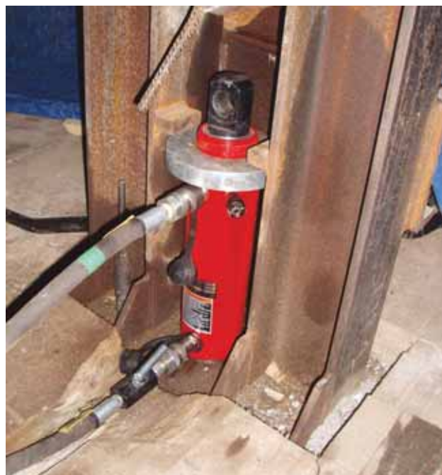
HD cylinders can be used in pushing and pulling applications. In this photo, we see a HD2506 HD cylinder set up for a pull application using a Plunger Clevis cylinder accessory
