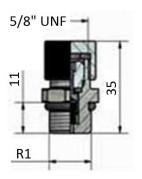
Nitrogen valve R:5/8" UNFBody of the nitrogen valve R:Zinc plated steel
