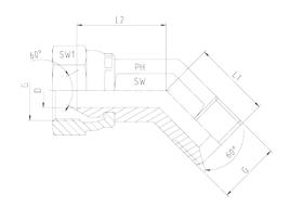
Male - BSP - Fixed with  $60^{\circ}$ -Cone Female - With Swivel Nut
