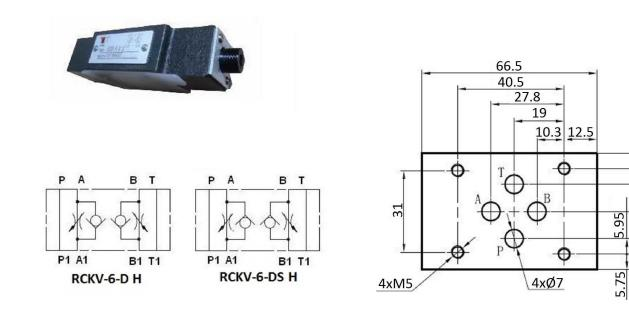
Operating Pressure 315 bar Flow Rate 80 l/min 4 Screw Set Included M5x85 Length=142 mm, Height= 28,6 mm Cast iron body
