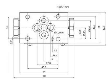
Max. Working Pressure 315 bar Opening Pressure 0,5 bar
