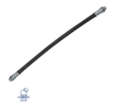
Length 300mm (12in) **Thread** 1/8in BSP Max. Pressure 15,000psi Material Rubber
