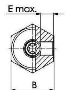
Material Body in Steel Cracking Pressure 0,5 bar
