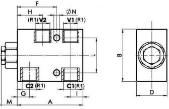
MaterialBody in AluminiumCracking Pressure2,5 bar (5bar and 10bar on request)
