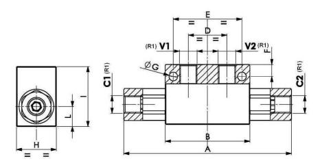
Material Body in Steel Cracking Pressure 2 bar
