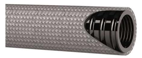
·Inner tube: convoluted tube in PTFE, resistant to fire, chemically inert. Suitable for food use, ·Reinforcement: stainless steel AISI 304 braid. Composition:
