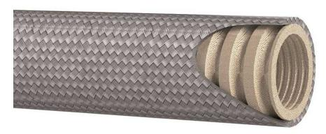
·Inner tube: convoluted tube in PTFE, resistant to fire, chemically inert. Suitable for food use, according to FDA norm.+ fiberglass band ·Reinforcement: stainless steel AISI 304 braid. Composition:
