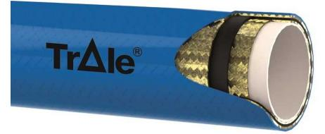
Composition: •Inner tube: polyamide PA6 •Reinforcement: two braids of steel wire. •Cover: blue polyurethane.
