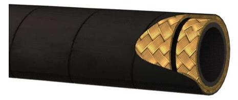
·Inner tube: special synthetic rubber resistant to hydraulic oil. ·Reinforcement: two braids of steel wire. Composition:
