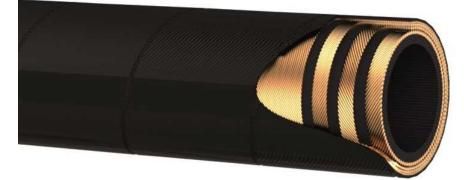
**Composition:** Inner tube: special synthetic rubber resistant to mineral, vegetable and hydraulic oil. Reinforcement: four braids of steel wire. Cover: synthetic rubber, very high resistant to oil, abrasion and weather.
