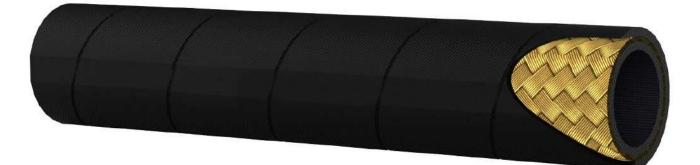
**Composition:** Inner tube: synthetic rubber resistant to hydraulic, mineral and vegetable oil. Reinforcement: one braid of steel wire. Cover: synthetic rubber resistant to oil, abrasion and weather.
