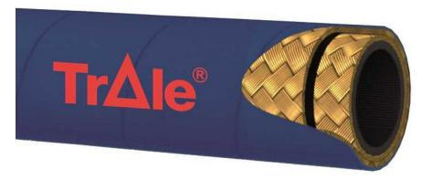
·Inner tube: special synthetic rubber resistant to mineral, vegetable and hydraulic oil. ·Reinforcement: two braids of steel wire. ·Cover: synthetic rubber resistant to oil, abrasion and weather. Composition:
