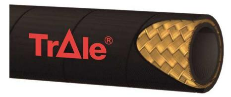
·Inner tube: synthetic rubber resistant to hydraulic, mineral and vegetable oil. ·Reinforcement: one braid of steel wire. ·Cover: synthetic rubber resistant to oil, abrasion and weather. Composition:
