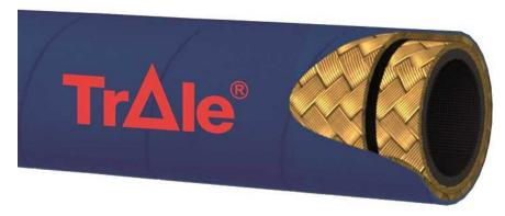
·Inner tube: special synthetic rubber resistant to hydraulic oil. ·Reinforcement: two braids of steel wire. ·Cover: synthetic rubber resistant to oil, abrasion and weather. Composition:
