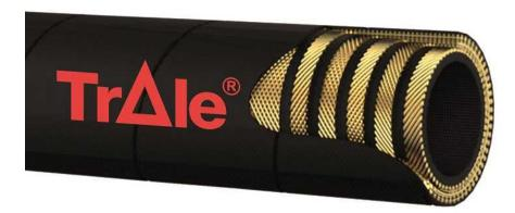
·Inner tube: special synthetic rubber resistant to mineral, vegetable and hydraulic oil. ·Reinforcement: 4-6 braids of steel wire. ·Cover: synthetic rubber, resistant to oil, abrasion and weather. Composition:
