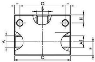
**Materials:** -body and internal parts are steel made. -external surface zinc plated.
