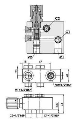
**Materials:** cartridges are in steel zinc plated, internal parts in hardened steel. Body is in high strength alluminium alloy.
