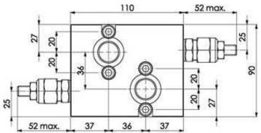
Cartridge is in steel zinc plated, internal parts are in hardened steel. Body is in high strength alluminium alloy. Materials:
