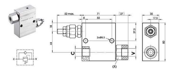
Material: Body in alluminium. Cartridge in steel zinc plated
