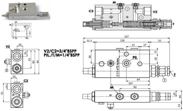
Adjustable pressure range (bar): 3,5-19,5 Pressure increase (bar/turn): 3,5 Standard setting (bar): 7,5 Spring valve 1
