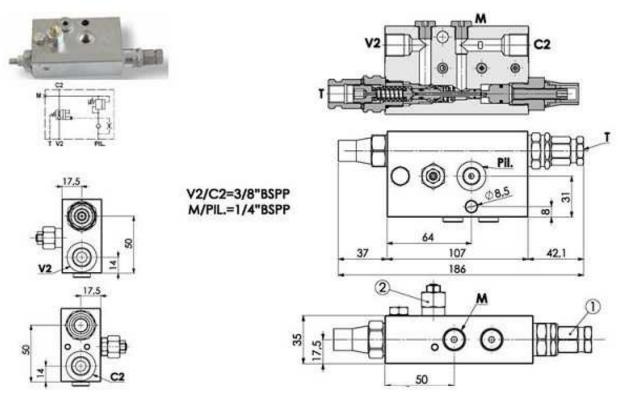
Adjustable pressure range (bar): 4-15,5 Pressure increase (bar/turn): 4 Standard setting (bar): 7,5 Spring valve 1
